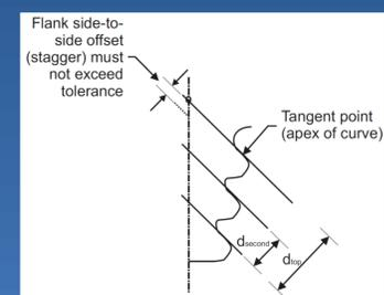
Illustration showing measurement location in cross-section
